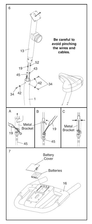
8. While a second person holds the Console (16) near the Upright (13), connect the console wire to the Extension Wire (52). Then, insert the wires downward into the Upright.
